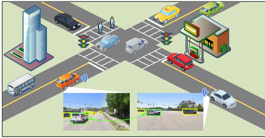
Figure 1: Collaborative perception example: two vehicles share sensory data to remove blind spots of each other, based on commonly visible (co-visible) objects in their views [12].
